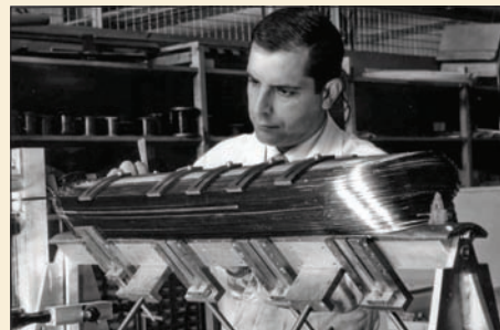
A full-scale copper-wound model of a pole produced at CERN to develop the coil-winding technique.
